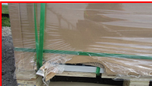
Forklift damage on pallet with exposed modules
